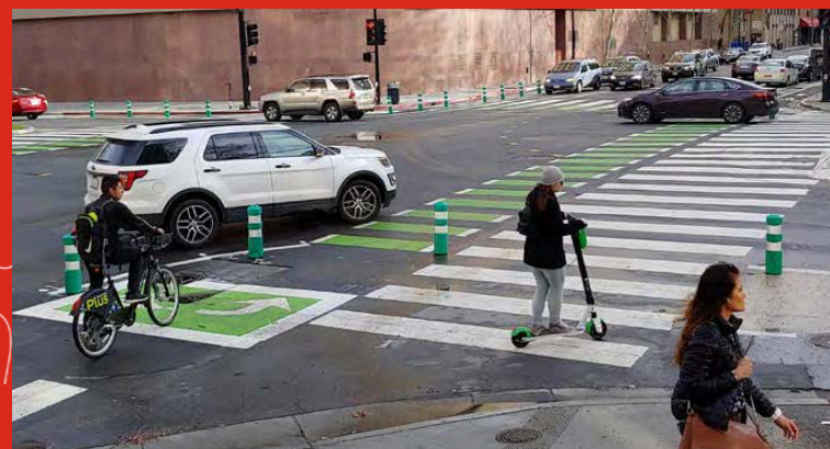
Turn hardening accommodates kinetic energy forces.
